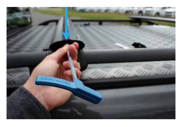
Apply downward force to the Cross Bars and push it down onto the side rails
