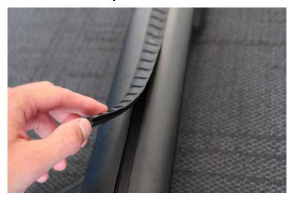
Push the rubber infill into the channel on top of the bar
